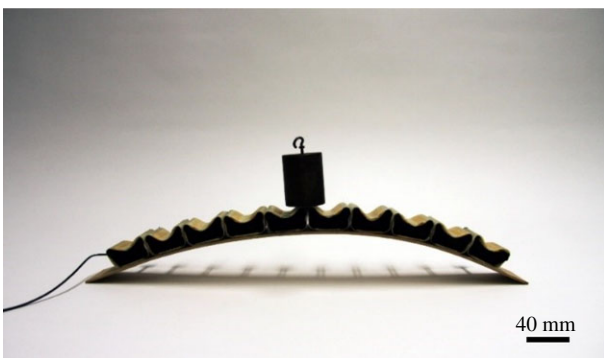
Figure 10. Physical prototype of the cellular actuator inspired by the bulliform cells of S. nitida . The structure lifts an external mass of 0.5 kg.
