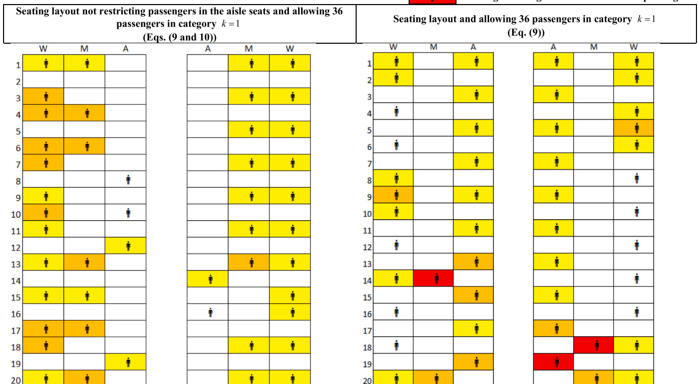
Fig. 8. Seat assignment to maximize the load of passengers using Eqs. (9 and 10).
