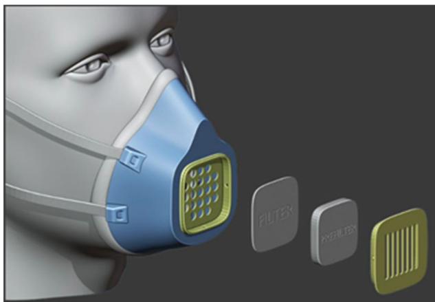
Fig. 10 COVID-19 mask by Lafactoria3d made of PLA [43]
