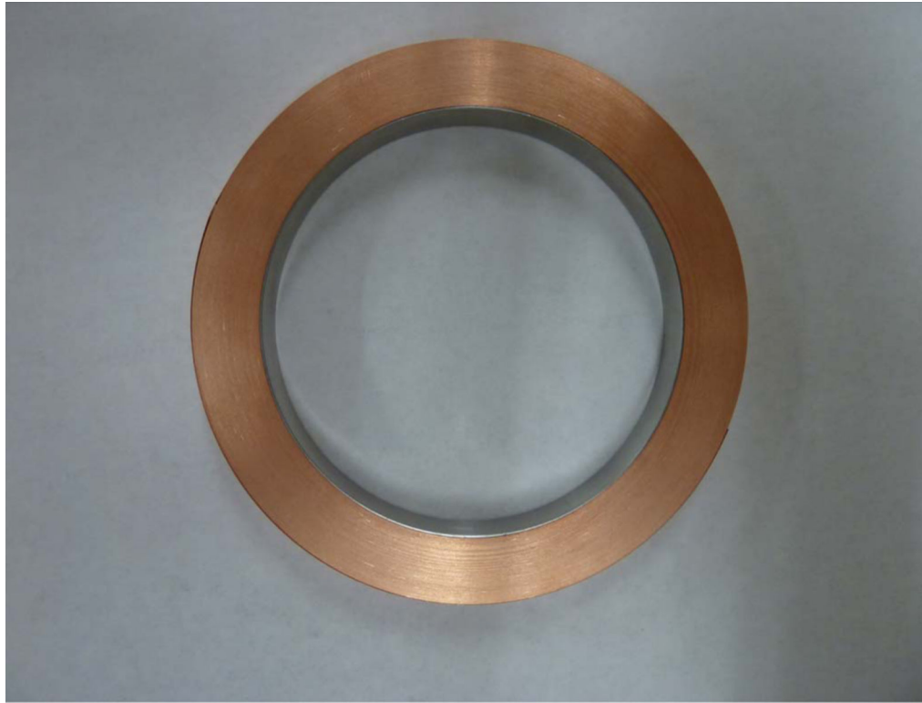
Fig. 4. Photograph of a completed DP coil showing the internal nonmagnetic stainless steel support ring.
