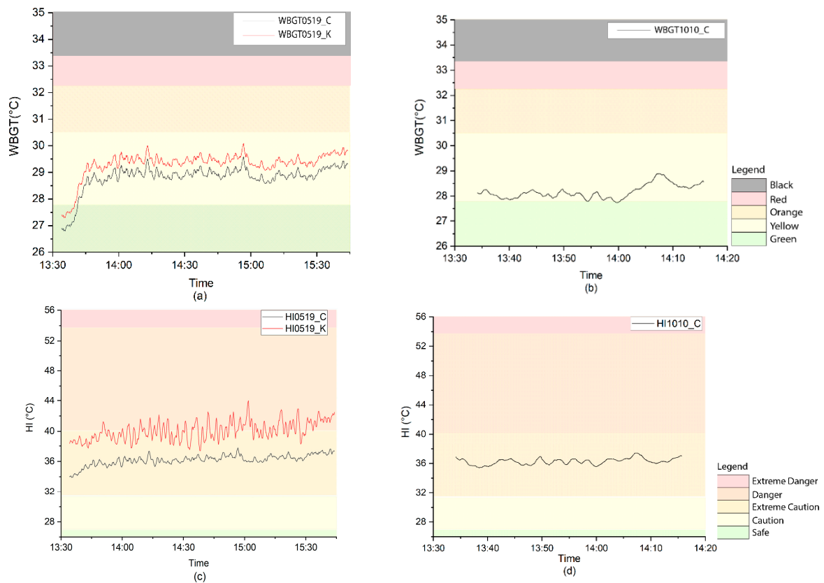
Figure 1. (a) Calculated WBGT heat stress and Kestrel WBGT on 19 May 2020; (b) calculated WBGT on 10 October 2019; (c) calculated HI heat stress and Kestrel HI on 19 May 2020; (d) calculated HI on 10 October 2019.
