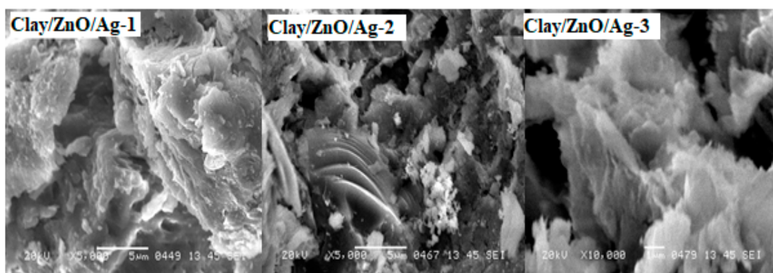
Figure 12. SEM micrograph of clay/ZnO/Ag-1, clay/ZnO/Ag-2 and clay/ZnO/Ag-3.
