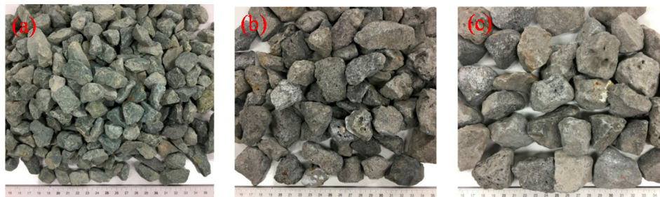
Figure 2. Photographs of the three different sizes of aggregate: (a) Small, (b) Medium, (c) Large.
