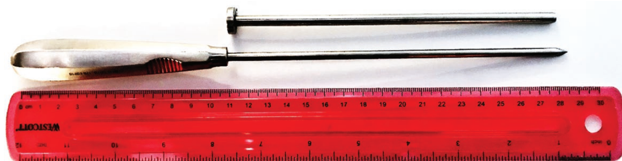
Figure 1. The custom biopsy instrument (SurgiPro, Minneapolis, MN) consisted of a sharpened trocar and cannula with a working shaft length of 17.5 cm and a cannula diameter of 6 mm. The combined instrument was inserted through the 11th intercostal space of the animal until the hepatic membrane was pierced, then the trocar was withdrawn, the cannula was inserted into the liver tissue, and the exterior opening of the cannula was covered as the instrument was retrieved from the animal. The negative pressure created by covering the exterior opening aspirated approximately 0.4 g of the liver tissue.
