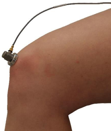
Figure 5. The accelerometer attachment: 1 cm above the apex of patella.
