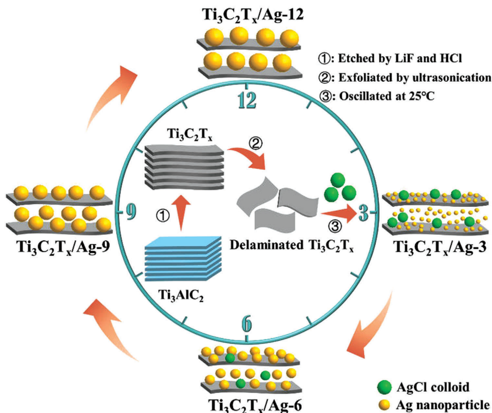
Figure 1. Schematic preparation of \text{Ti}_3\text{C}_2\text{T}_x/\text{Ag} samples.
