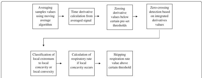
Fig. 5 Signal processing pipeline for BarTek device. Real-time signal processing is based on a zero-crossing algorithm with further modifications. It is important to note that zero-crossing detection is based on a dynamically adjusted threshold. The basic signal processing algorithm consists of seven steps
