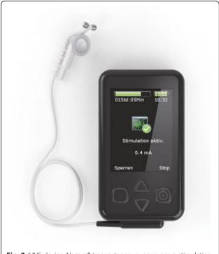
Fig. 2 tVNS device. Nemos® transcutaneous vagus nerve stimulation (tVNS) device (Figure taken from [69])
