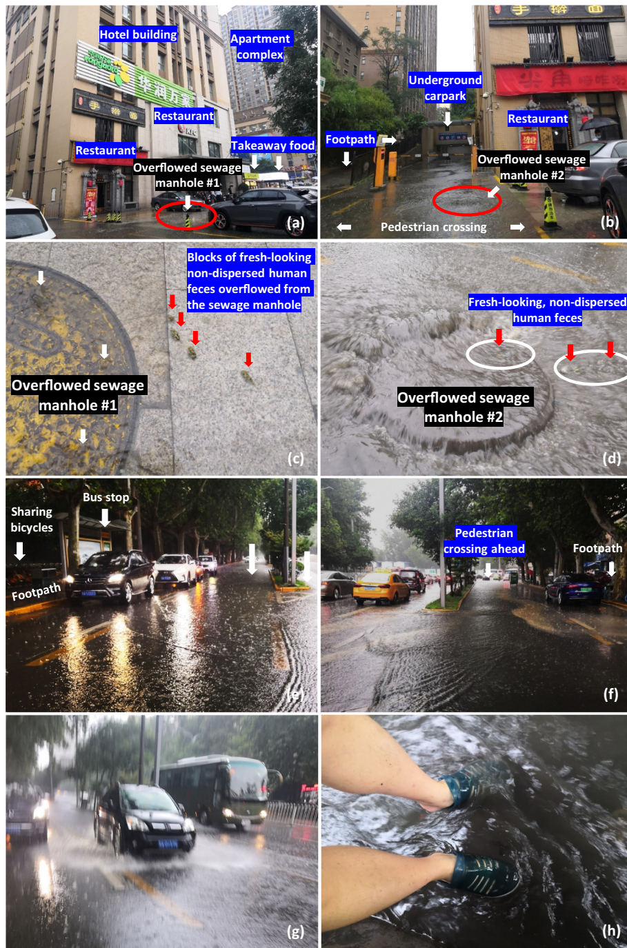
Fig. 2. Combined sewer overflows (CSOs) from manholes during an urban flooding event in Xi'an, China on July 30, 2020. (a) (b) Locations and surrounding environments of two overflowed sewage manholes (red circles); (c) (d) close-up pictures of the manholes, where blocks of fresh-looking, non-dispersed human feces were visible in CSOs and on adjacent ground (red arrows); (e) the CSOs flew to lower grounds, causing flood on an adjacent street; (f) the dark-colored CSOs continued for several hundred meters down the street, and mixed with stormwater runoffs from a nearby construction site; (g) splashes and aerosols of the CSOs generated by vehicles driving through the flooded area; (h) direct skin contact with the CSOs by a pedestrian walking across the street.
