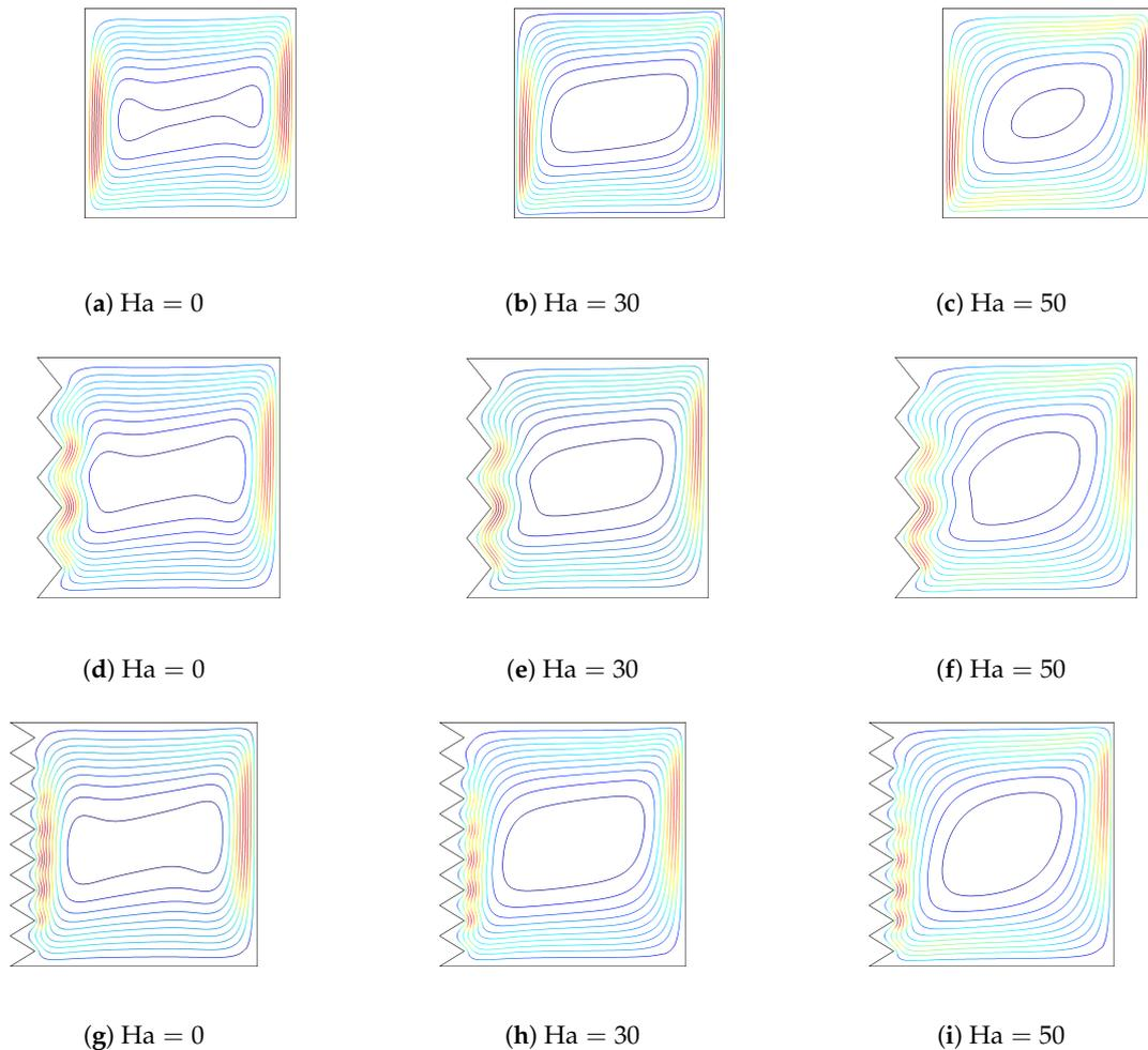
**Figure 7.** The effect of varying the Hartmann number on the streamlines for flat and corrugated walls ( $Gr = 5 \times 10^4$ ,  $Da = 10^{-2}$ ,  $\phi = 0.02$ ).
