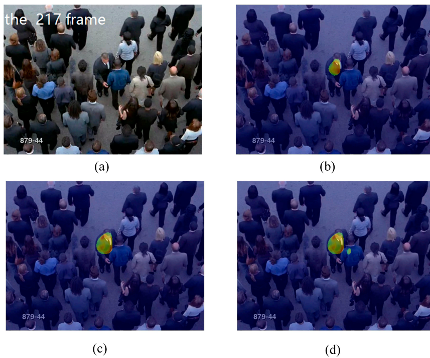
Figure 10. Retrograde motion detection in single retrograde scene using different neighborhood size: (a) original video frame; (b) detection result using 5 \times 5 neighborhood; (c) detection result using 15 \times 15 neighborhood; (d) detection result using 23 \times 23 neighborhood.
