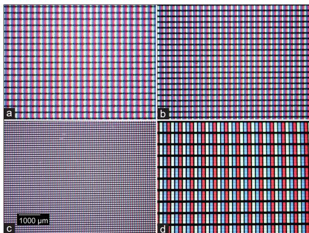
**Figure 4:** Relative pixel density and size of different display resolutions: (a) Dell MR2416 (24", 1920 × 1200) (b) Philips PP27QHD (27", 2560 × 1440) (c) Apple Pro XDR (32", 6016 × 3384) (d) Samsung QM85D (85", 3840 × 2160). All at effective × 59. As can be seen in a-c, pixels generally decrease in size as resolution increases, however this is offset by the relative screen size (d)
