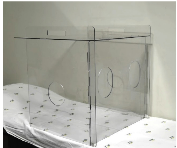
Figure 2. Aerosol chamber demonstrating the different holes.
