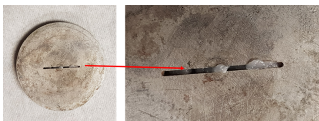
Figure 9. Aluminum fractured disc ( 1'' \times 1000 \mu\text{m} ) completely sealed with PAM/AlAc (9:3).
