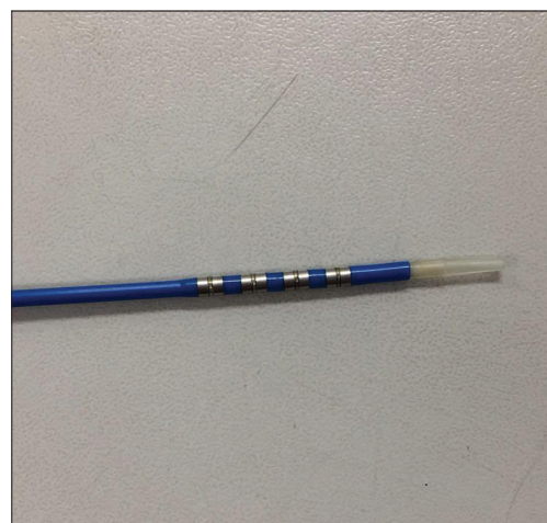
Figure 1. ELRA radiofrequency catheter with an 18 mm active segment made of four stainless circumferential ring electrodes (width 3 mm) spaced 2 mm apart
