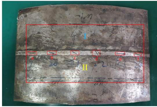
Figure 17. Pipe piece with weld defect. (Online version in colour.)
