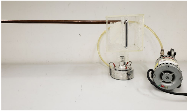
FIGURE 6 The copper tube-acrylic box sampling manifold
