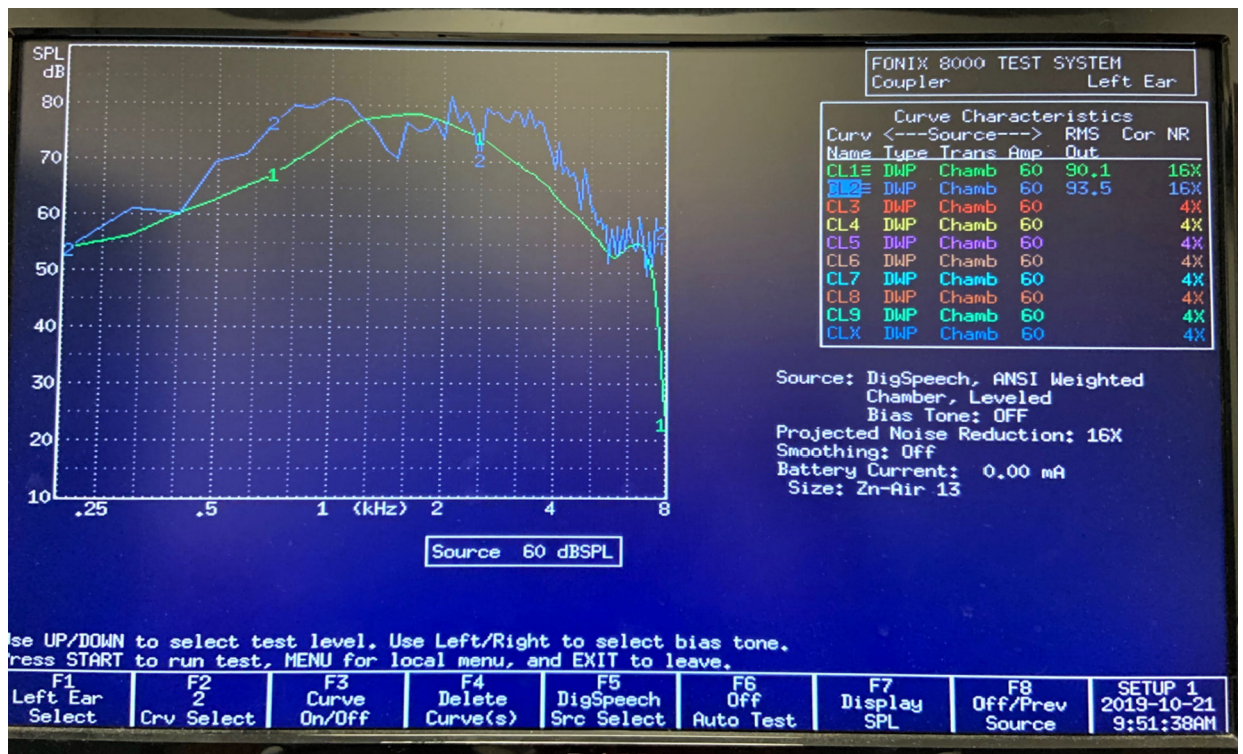
Fig. 5: Comparison of hearing aid output with developed smartphone application on Fonix 8000 hearing aid analyzer. Curve 1 (green) represents the output of the smartphone-based hearing assistance, and Curve 2 (blue) represents the output of a Starkey Halo Hearing aid
