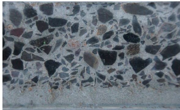
Figure 1. The structure of spun concrete in the wall thickness of a power pole.
