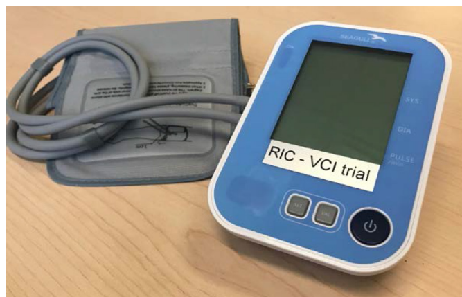
Figure 2 Device for applying remote ischaemic conditioning (Seagull Apps, Denmark). The device applies four cycles of remote ischaemic conditioning on pressing the button. Device activations are recording, including the number of cycles. Systolic blood pressure, diastolic blood pressure and pulse are displayed.
