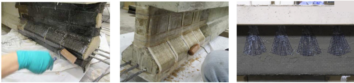
Figure 9. End anchorage system using CFRP or glass FRP (GFRP) strips [28], and plugs of fan-shaped CFRP anchors inserted into holes inside the concrete surface [7].
