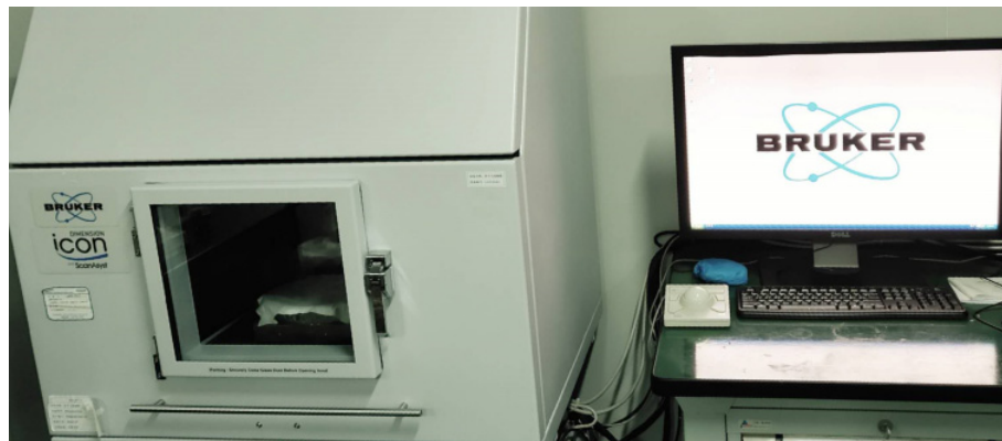
Figure 6. Atomic force microscope (Bruker Dimension Icon). The results showed that the roughness values were small after processing (Figure 7).
