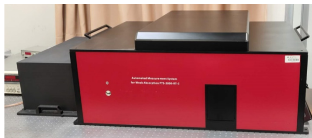
Figure 11. Photothermal weak absorption test platform.
