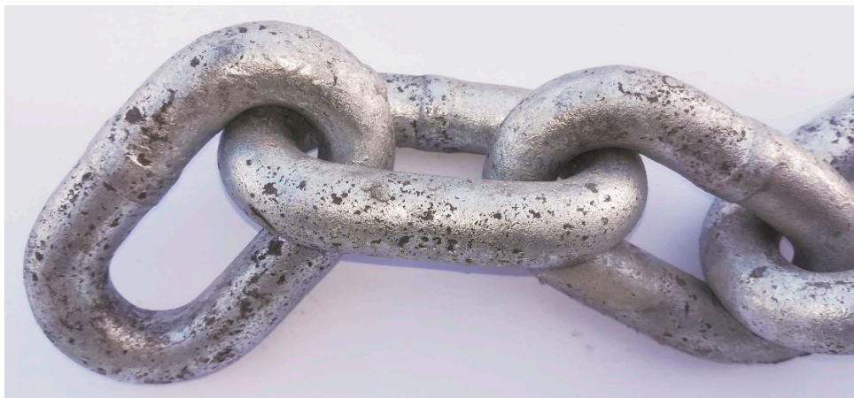
Figure 1. The appearance of the chain surface with a zinc coating obtained in a bath containing an excessive amount of Al (0.25 wt % Al); chain size 18 × 64 (photo by H.Kania).
