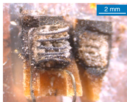
Figure 2. Stereozoom microscope image of dissected, cylindrical ceramic heating element from the vaping cartridge of a patient with electronic cigarette, or vaping, product use-associated lung injury, showing charring from high temperatures. Scale bar, 2 mm.
