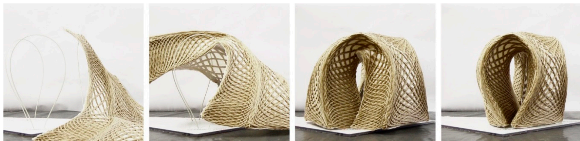
Figure 11. Process of placing a preform on bent scaffolding rods.
