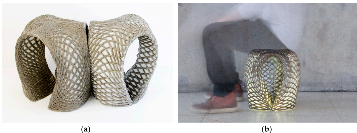
Figure 17. Possible connection of two components (a), prototype in use with integrated lighting (b).
