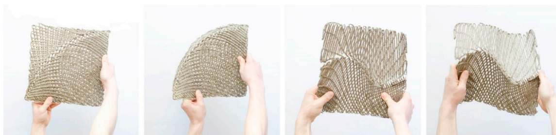
Figure 16. Sample 1 (left) and sample 2 (right) with compliant curved hinges.
