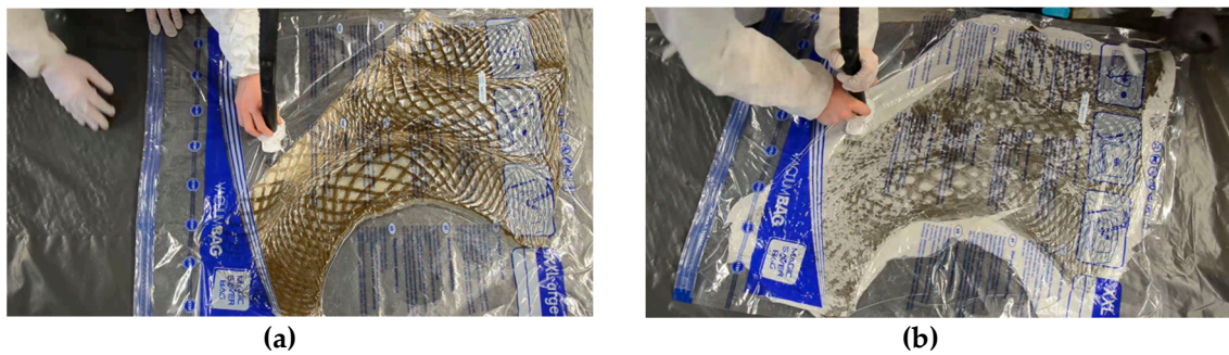
Figure 10. Resin vacuum infusion process (a), removal of excessive resin with a sacrificial material (b).
