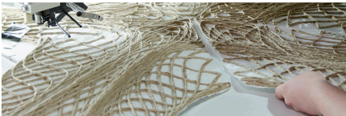
Figure 14. Placing the last fifth of the third prototype on the TFP machine for the connection.
