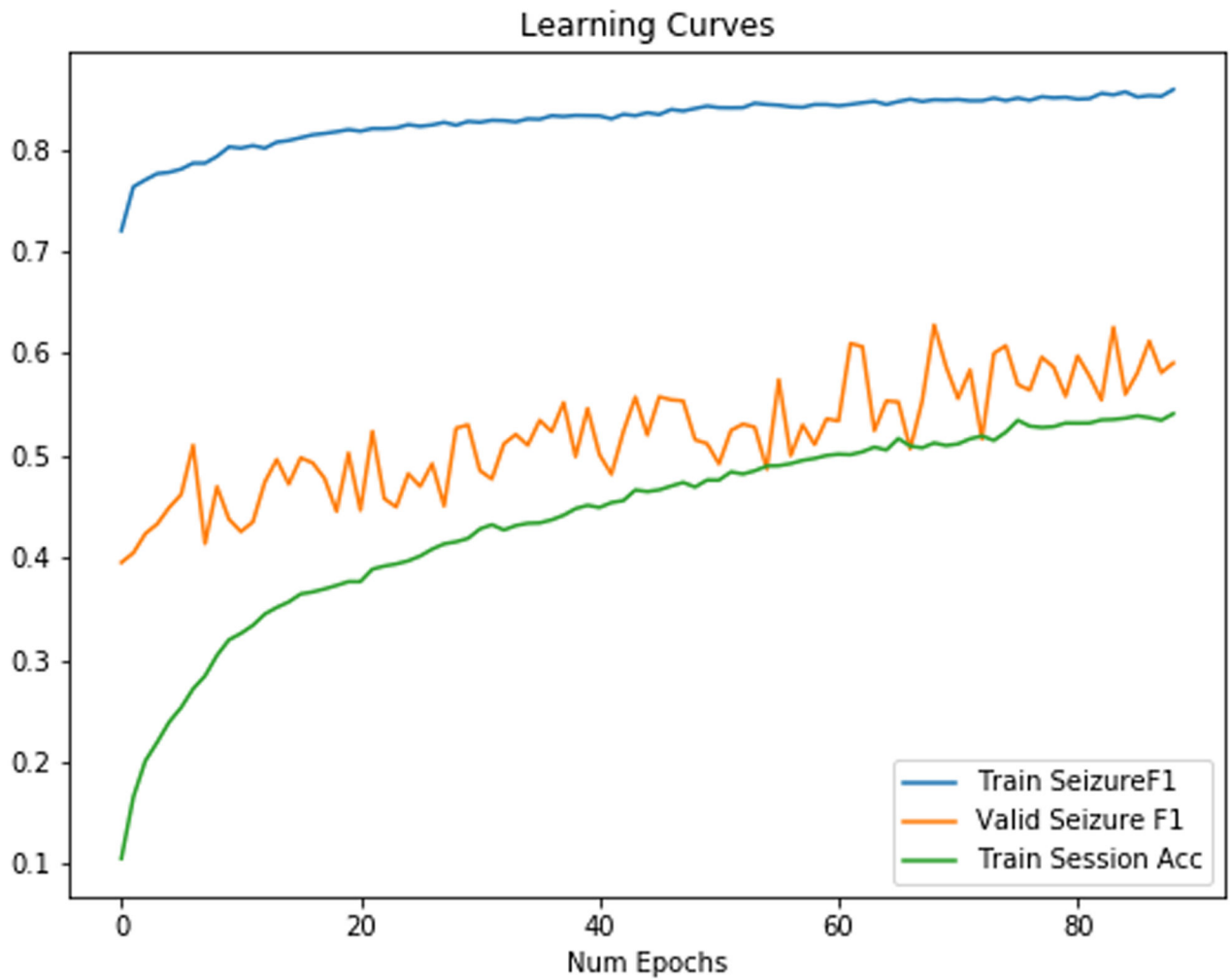
Figure 10: Training/Validation F1 Score for a neural network with randomly rearranged channels on each minibatch and random rescaling on each minibatch of 2. There is a monotonically increasing training session identification again.
