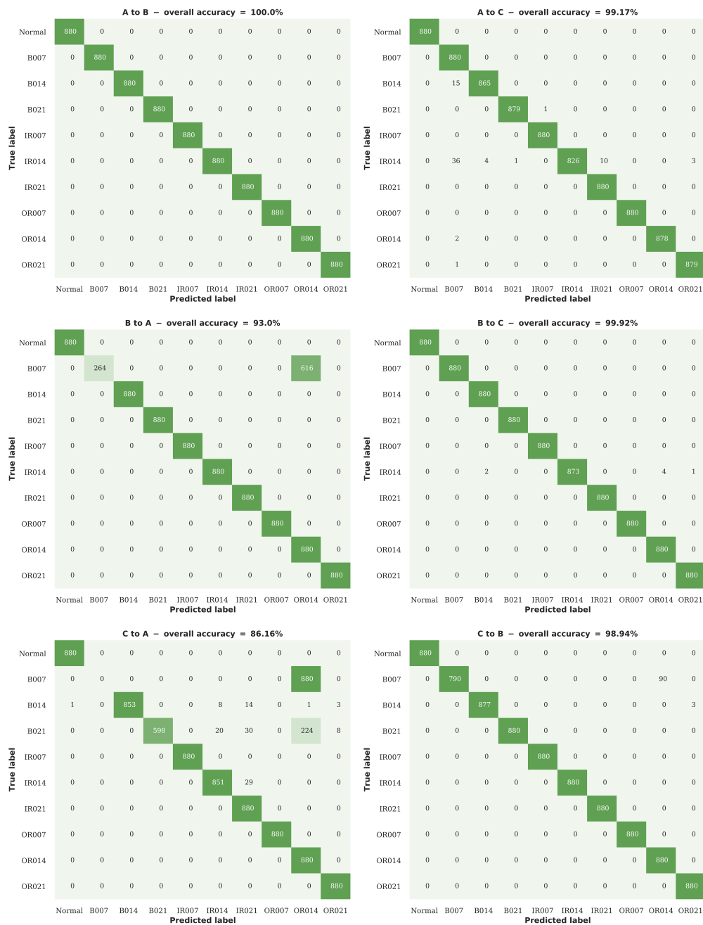
Figure 9. Confusion plots for the RNN-WDCNN model on the 6 different domain adaptation cases considered in scenario 1.
