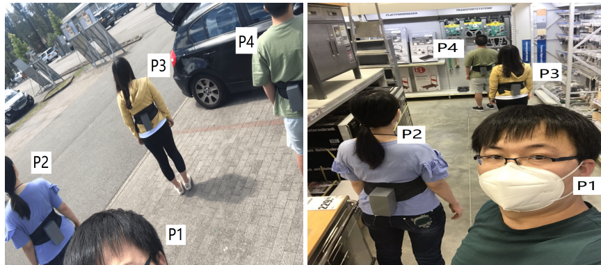
Figure 19. Four volunteers' practical test outside and inside the construction material supermarket where a more complex environment exists. P1 and P2 as one group with a distance of 1.0 m and P3 and P4 as another group with a distance of around 1.5 meters, the distance between the two groups is beyond 3.0 m.
