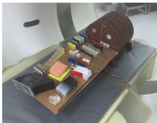
Fig. 2 Multiple samples were assembled on Siemens Somatom Definition AS+ scanner with an ACR phantom used for scanner calibration. The scans were repeated for multiple kVs and ROIs were measured to determine the CT number of each sample
