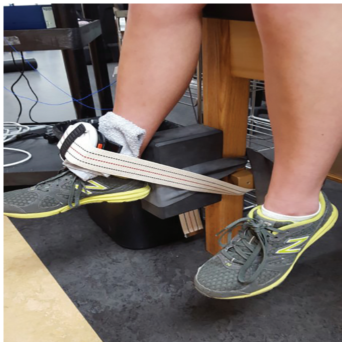
Figure 2. Collection of knee extension force data utilizing a handheld dynamometer.
