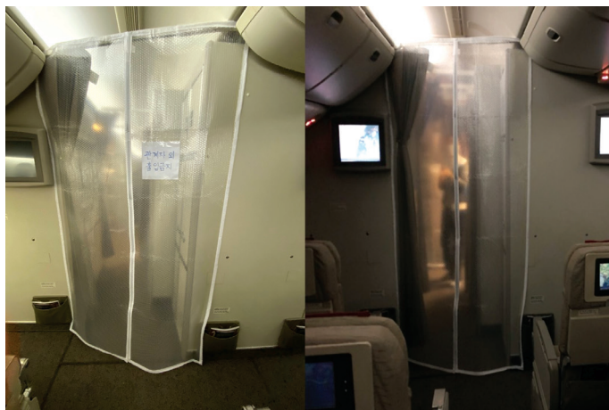
Figure 2. Vinyl curtain doors. The doors were attached with a double-sided adhesive tape. The center contains a magnet, so when people push, the magnetic door opens, and closes automatically.
