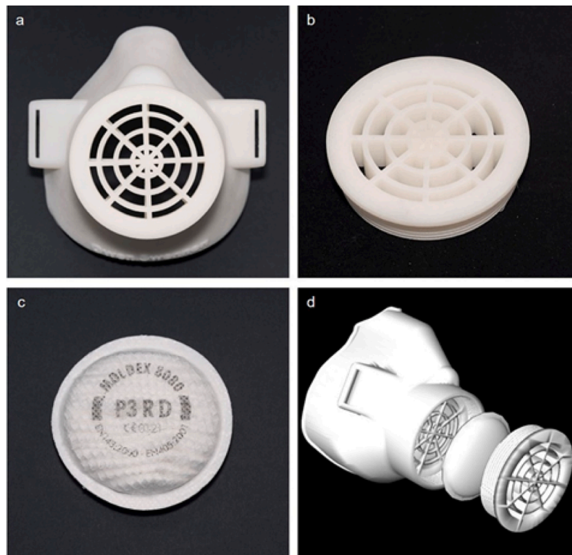
Fig. 15. (a) Custom-made individualized 3D printed protective face mask, (b) filter membrane for support, (c) polypropylene (PP) non-woven melt-blown particle filter, (d) Three-Dimensional image of the prototype [54].
