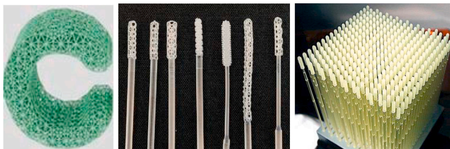
Fig. 6. Lattice structures of the 3D-printed antibacterial bio-cellulose swabs were produced for the COVID-19 test [34–38].
