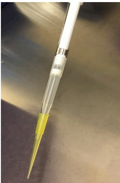
Figure 7. Put a p200 Tip on Top of a p1000 Filter Tip to Disrupt the Organoid Structures
