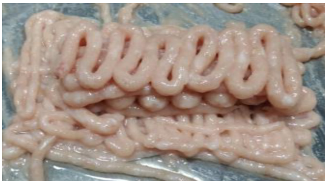
Figure 4. 3D-printed cooked-meat slurry with 100g water and 40g gelatin powder added. Picture taken from an article by Liu et al. [12]
