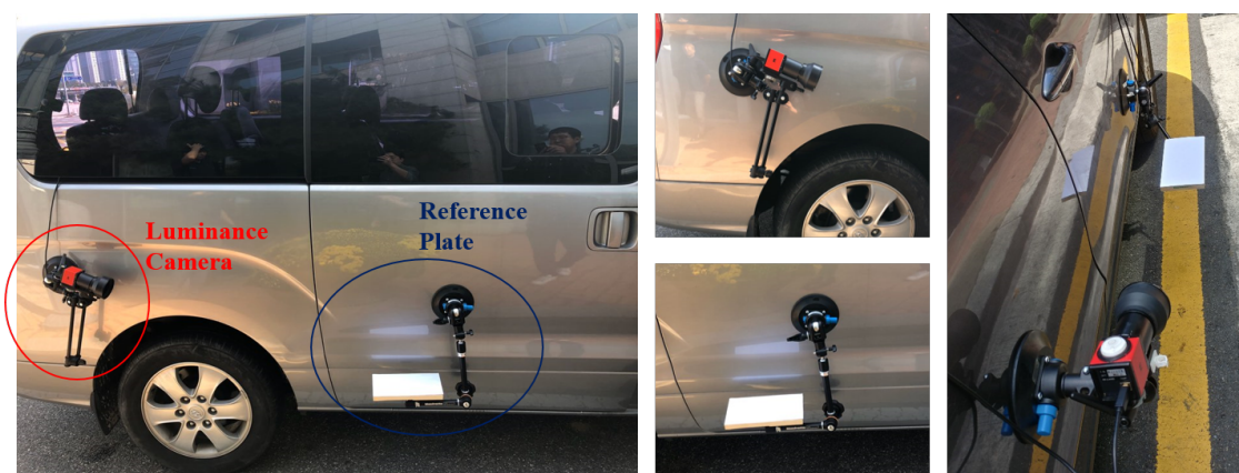
Figure 3. Placement of the luminance camera and reference plate on a vehicle used to capture luminance images.
