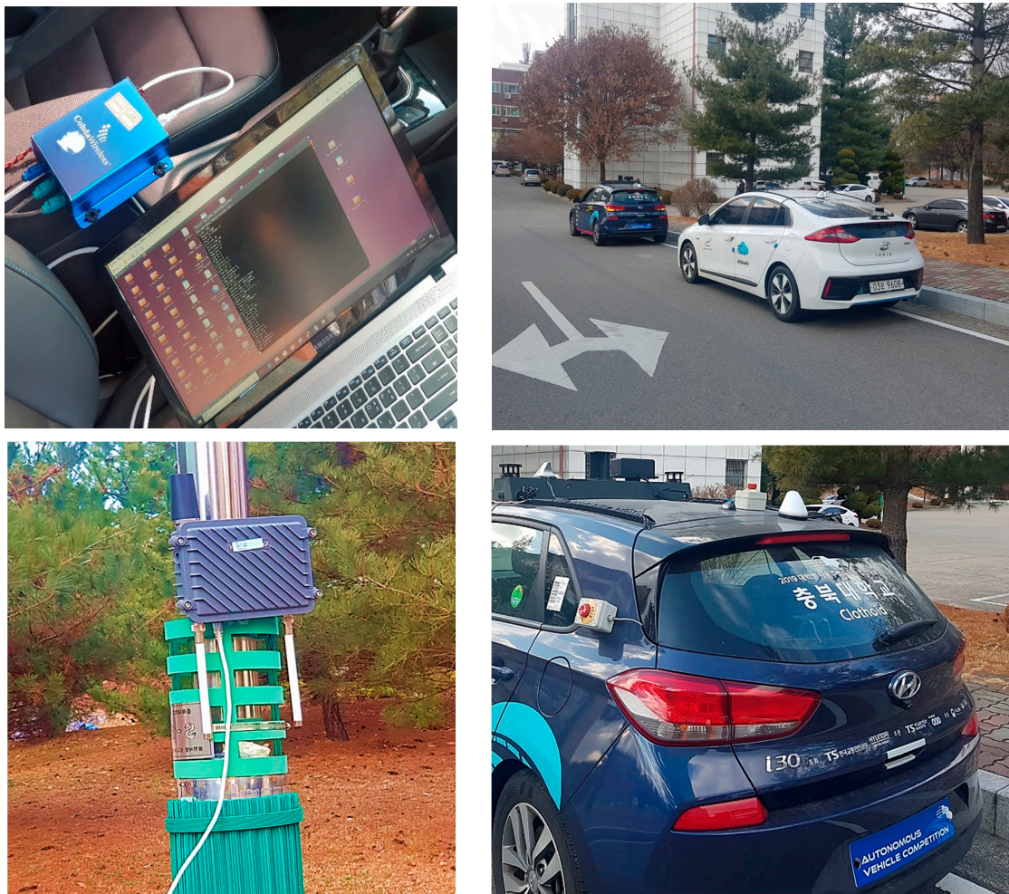
Figure 10. Our test platform consisting of test vehicles, GPS antenna, MK5 OBU devices, and RSU devices.
