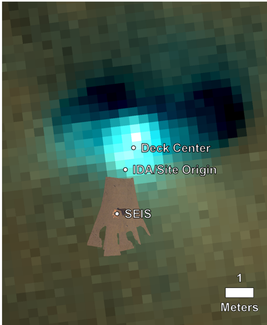
Figure 9. Georeferencing the IDC orthophoto of the workspace from the IDA stereo images and DEM onto the HiRISE image ESP_057939_1845_RGB using the translation from the deck center to the site frame origin. The distance between the center of the spacecraft and the SEIS location is 2.42 m.
