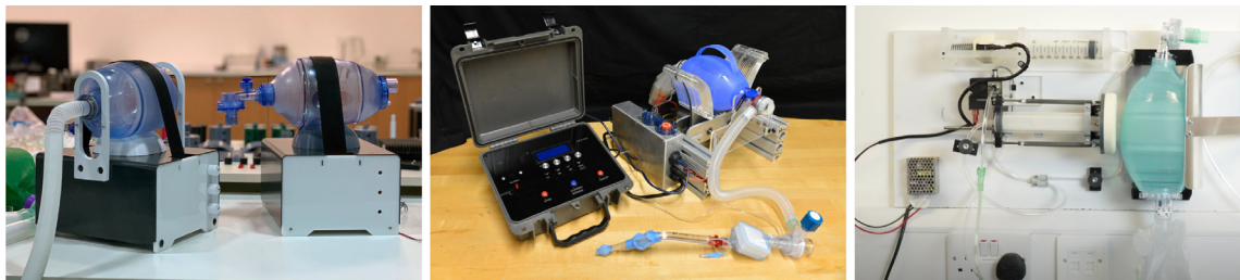
Fig. 3. Different approaches for automating the squeezing of an AmbuBag, via pulleys (VentCore, left), motorized claws (E-Vent, center), pressurized air (Gtech, Right).
