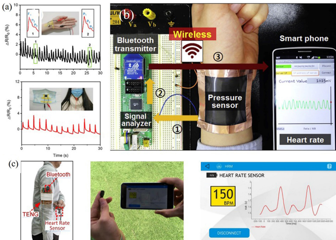
Fig. 10. (a) Wearable sensors for monitoring wrist activity and breathing during sports [84]; (b) Wireless sensor for heart rate monitoring through the wrist [85]; (c) BSN system application demonstration [86].
