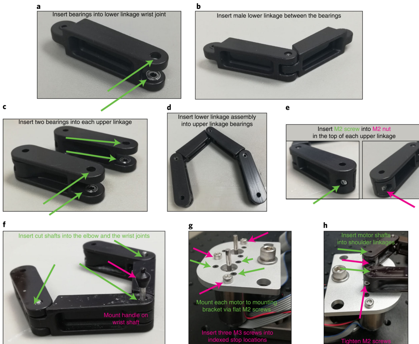
Fig. 2 |. Detailed manipulandum assembly.
