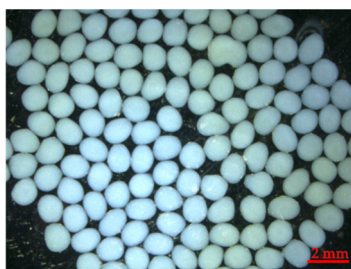
Figure 3. The encapsulation of crude dextranase from Penicillium roquefortii TISTR 3511 in alginate beads.
