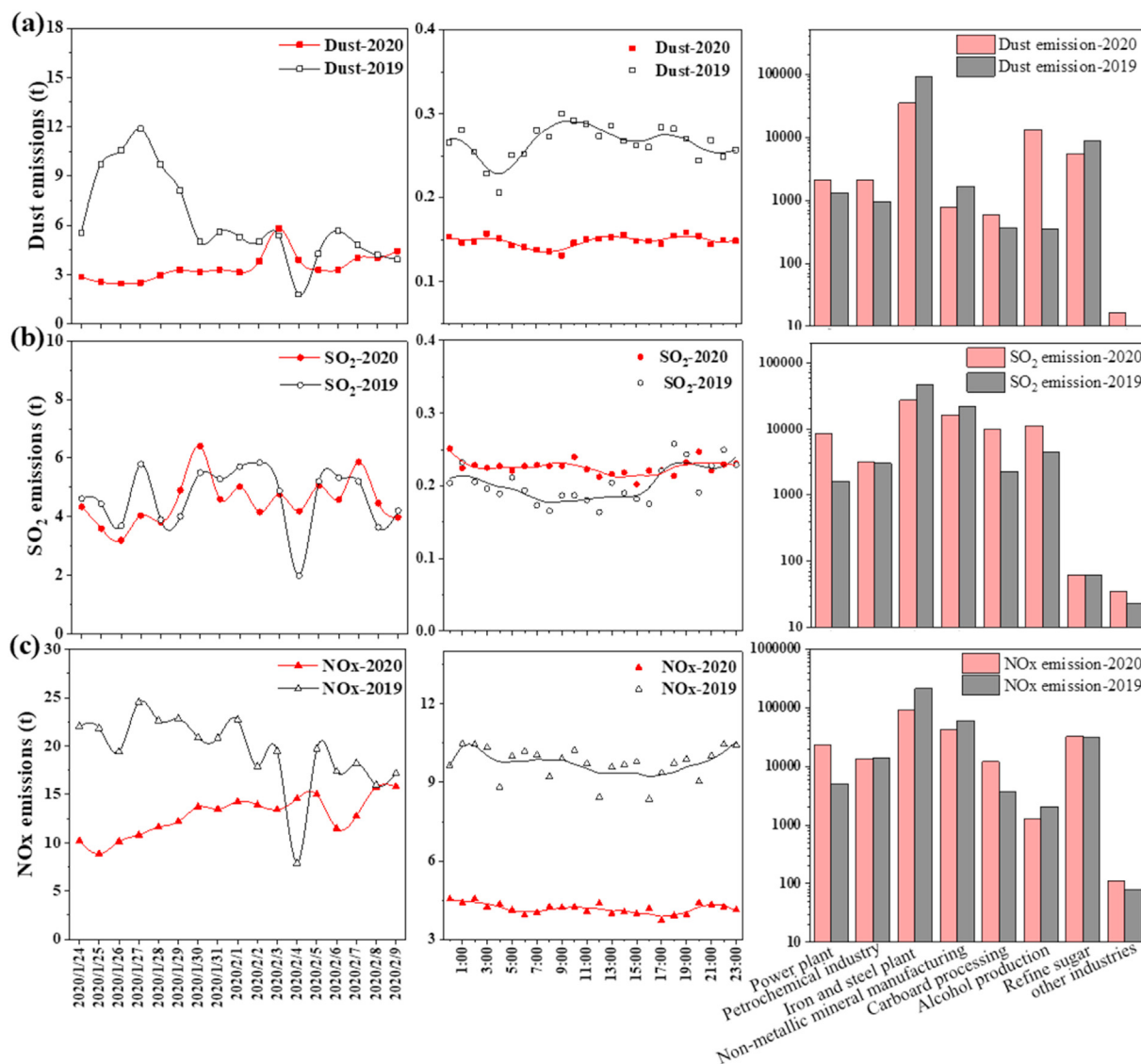
Fig. 5. Emission variations of dust, SO 2 , and NO x observed by CEMS during lockdown period.
