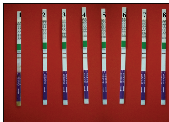
Figure 5. Cry1Ac protein expression in transgenic sugarcane on QuickStix Combo strips. Lines 6 and 8 showed negative results (one band). Lines 1, 2, 3, 4, 5, and 7 showed positive results (two bands).
