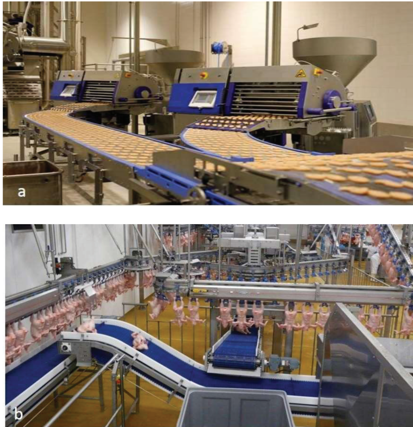
Figure 1. Modern fresh and processed meat plants (a) fully automated forming line, capable of producing 200,000 identical nuggets per hour; (b) in line automated sorting at a fresh poultry processing plant. Courtesy of Marel.
