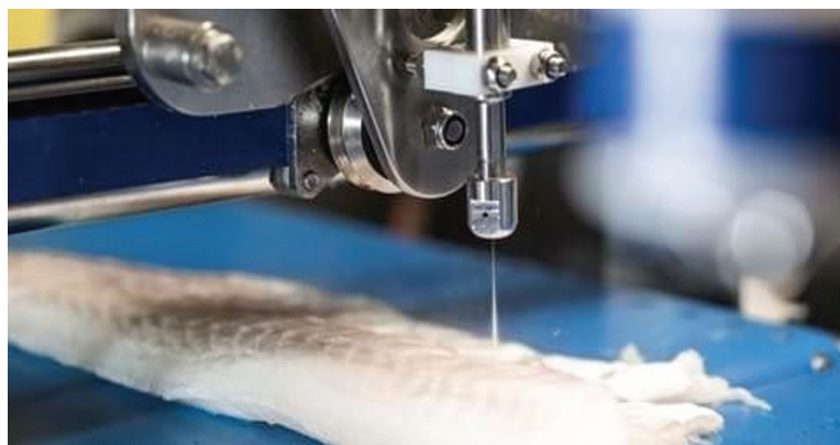
Figure 6. Automated fish trimming, using a water jet knife. Cutting pattern is controlled by a machine vision system. Courtesy of Marel.
