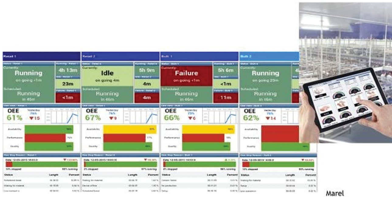
Figure 9. Real-time tablet presentation of the entire broiler primary processing plant. Data are collected from a wide range of sensors. Courtesy of Marel.
