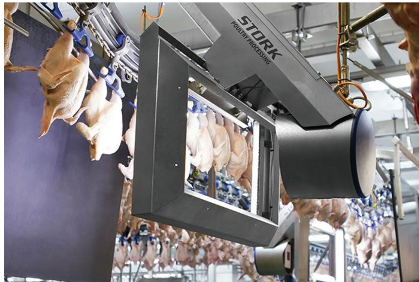
Figure 3. Image analysis system used to grade and sort broilers. Courtesy of Stork.
