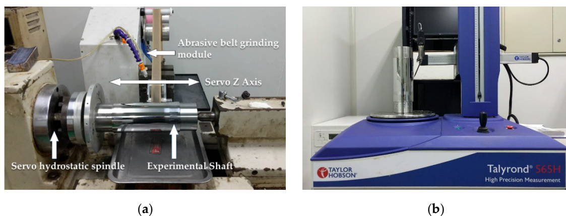
Figure 12. Actual figuring and measuring equipment of the experimental shaft: (a) modified lathe; (b) Talyrond™ 565H cylindricity meter.
