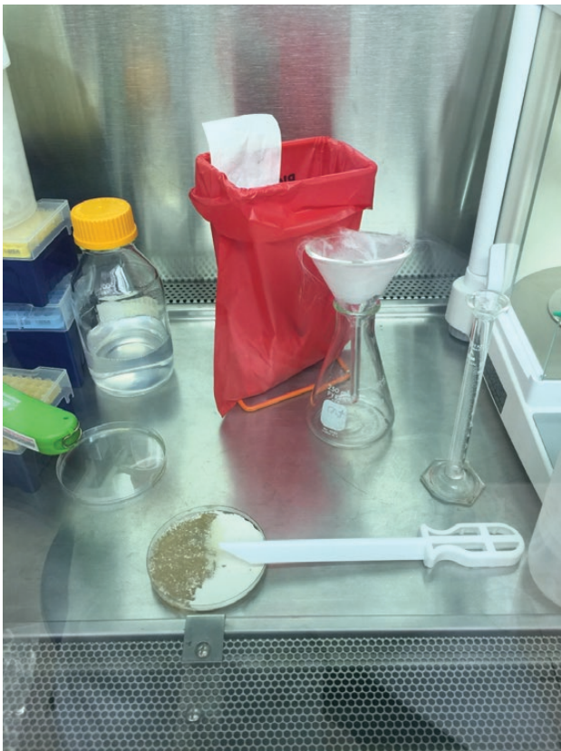
Fig. 3. Setup for wet harvesting of Beauveria bassiana from agar plates using 0.5% CapSil. The left side of the plate has been scraped with the sterile plastic disposable spatula shown.
